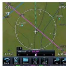
CDI indicates the OBS heading. The mode displays on the annunciator bar.
