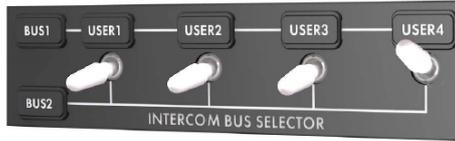
If one user is to be **ISOLATED** from the other users, that user must be connected to a different bus to all the other users. (i.e. User's switch must be in the opposite direction to all the others.) In this example, User 4 is isolated from Users 1, 2 and 3.
