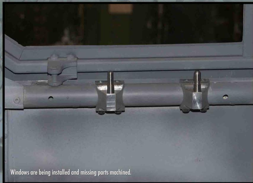
*Windows are being installed and missing parts machined.*
