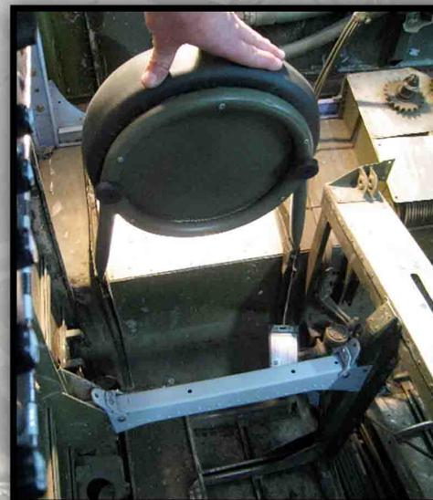
The navigator jump seat which sits on the starboard side of the pilot seat is ready to be installed. It's been cleaned, upholstered, primed and painted.
