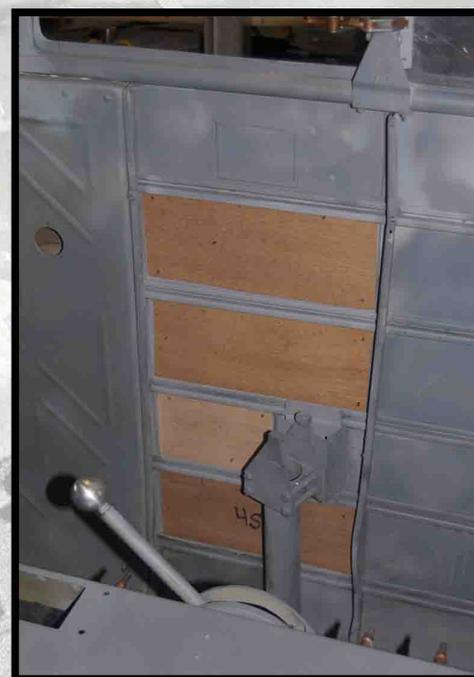
The wooden panels on each side of the front fuselage have been installed. They will need to be riveted and painted.
