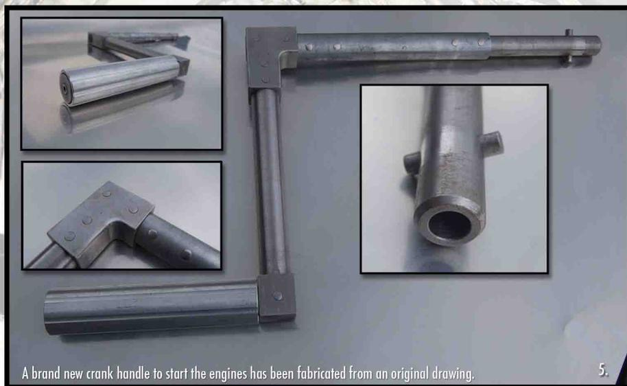
A brand new crank handle to start the engines has been fabricated from an original drawing.
