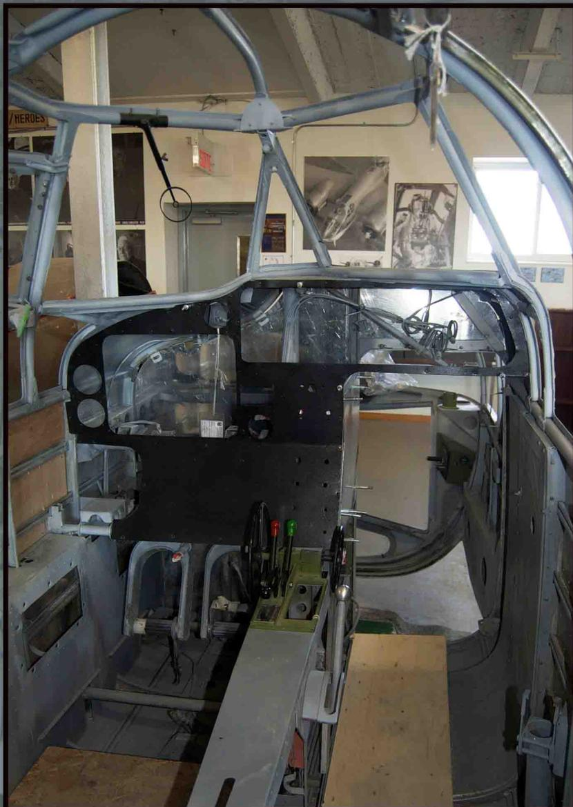
The main instrument panel has been fitted in place. A new panel had to be fabricated, the original panel being too damaged. The other panels will be installed soon. The rudder pedals leather straps will be replaced also. Part of the throttle quadrant has been temporarily installed. The hydraulic hand pump will have to be fabricated using drawings, pictures and measurements taken from different museums. The wooden floors will be one of the last items to be installed in the front fuselage.
