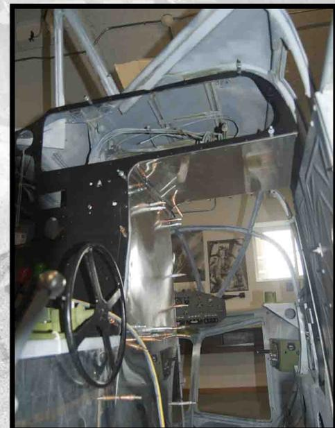
*Inside the forward fuselage as new skin panels have been installed.*
